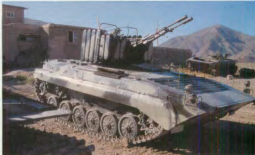
UF re-engineering job: a BMP-1 converted to carry the ever-popular ZU-23 twin cannon instead of the old 73mm smooth bore. The ZU-23 is far more effective in an anti-personnel role.
