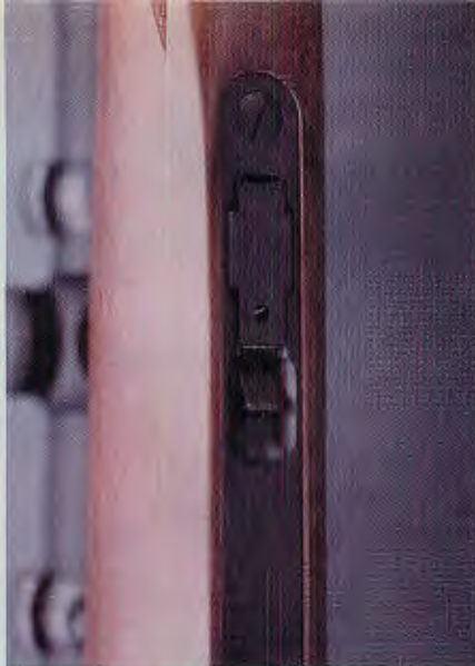
The five-round single-column magazine used by the Kimber Classic .22 rifle is flush mounted and retained by a spring steel latch. The bottom metal, as well as the triggerguard, are made from steel.
